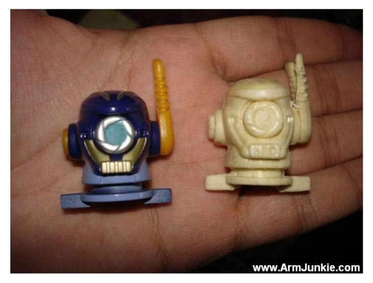
This is how the antenna came out due to the bad mold. I'm just going to cut it off and sand it. Other than that imperfection it was a good cast.
