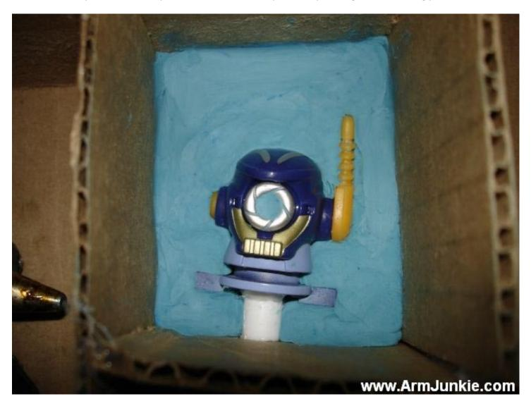
The clay must be as smooth as possible. Take special care to cover up any exposed edges around the object. Press in the eraser end of the pencil into the clay a few times. This will dimple the clay, making two interlocking pieces.
