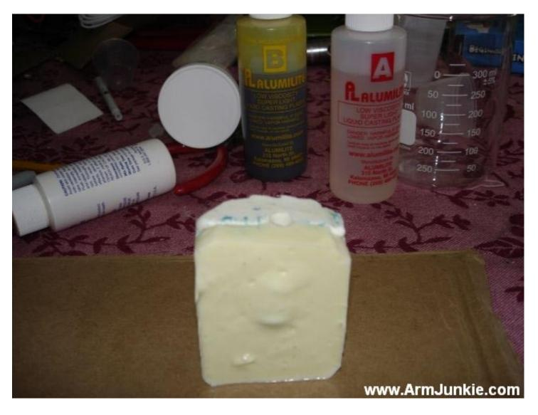
Once the second half of the silicone mold has hardened you can safely remove the robot head piece. You can extract both silicone halves from the cardboard holder.
