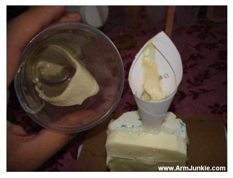
Here you can see how quickly the plastic hardened. It took the shape of the pour. Aside from the failure, that is pretty impressive.
