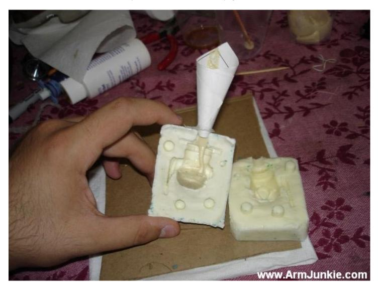
Now it is time to remove the failed attempt and clean out the mold to try again.
