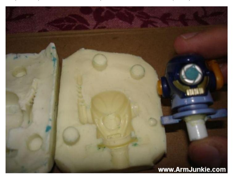
Here you can compare and contrast the robot head piece with the mold. A lot of detail is captured by the mold.
