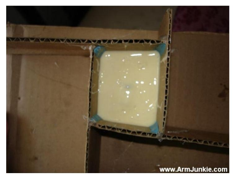
Once the silicone has hardened I removed the back of the cardboard mold. I carefully picked off the clay. Here is where I made my first huge mistake. I got overexcited and decided to remove the robot head to take a picture. This was a huge mistake because once dislodged, the piece would no longer fit snugly when placed back. This will produce a slightly warped piece and the "antenna" on the side will be completely ruined.
