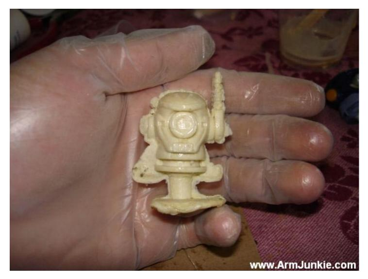
The mold did capture a lot of detail. Since I don't have any clamps on hand, I'm going to tape up the mold securely and try again.
