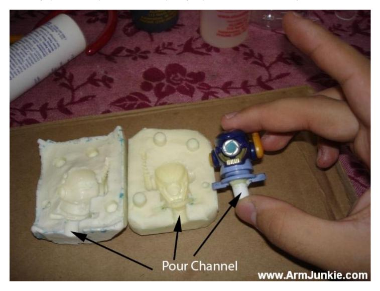
In this image, you can see the pour channel used for pouring the plastic resin into the mold cavity.
