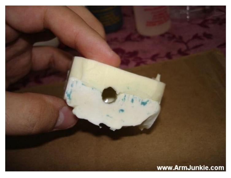
All things considered, it's a pretty good mold for a first timer. I can see that the mold won't be perfect. I got some air bubbles trapped due to not having my own vacuum chamber. I can see a problem with the robot's antenna. It must have moved during the mold making process. It doesn't look like the antenna will cast properly but let's continue anyway.
