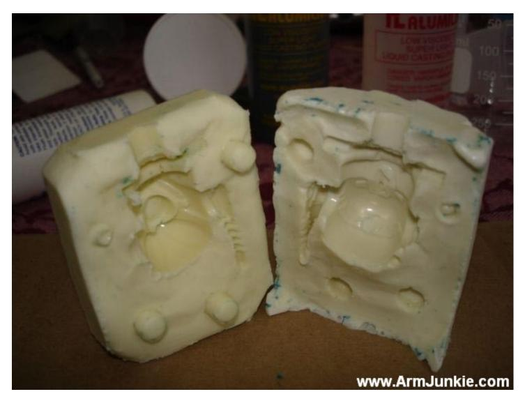
Notice how dimpling one side in the clay produced the interlocking teeth. Other than the botched antenna there were no serious mold deformations. You can spot two small air bubbles on the left edge of the left mold half in the following image.
